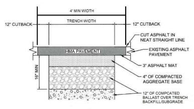
Note: For locations of existing asphalt mat thickness not equal to 3", match existing asphalt mat thickness.
